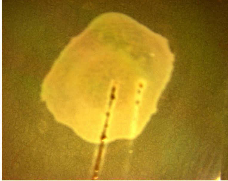
Figure 20. 0.50 and 0.35 W Laser Burn Lines through Spore Sample
