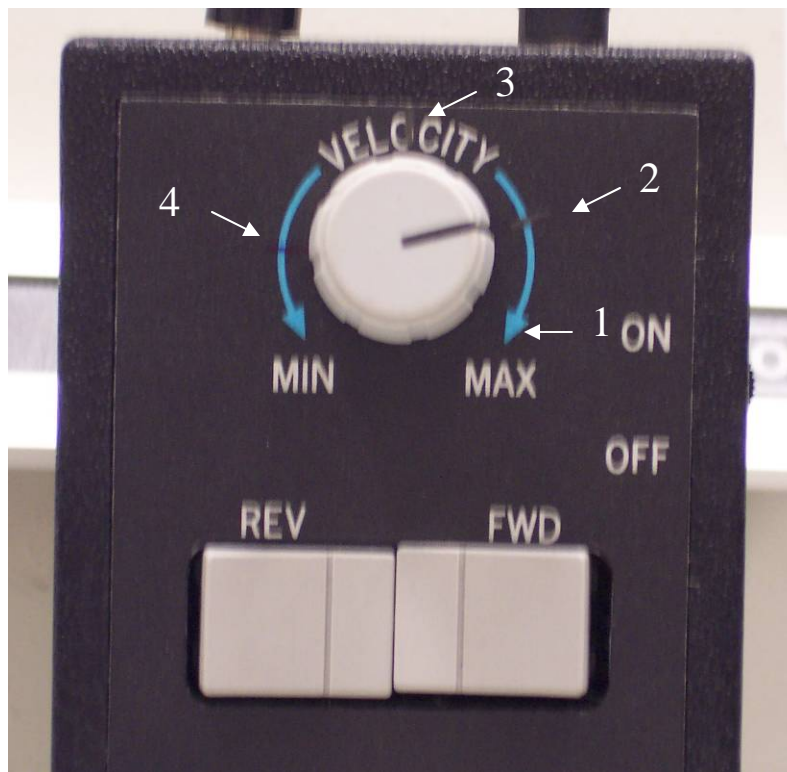
Figure 16. Handheld Sample Stage Controller for Bomem. Four velocity settings are marked with white arrows.
